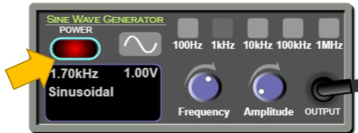
*Frequency knob:* You can rotate this knob to vary the value of the frequency.
