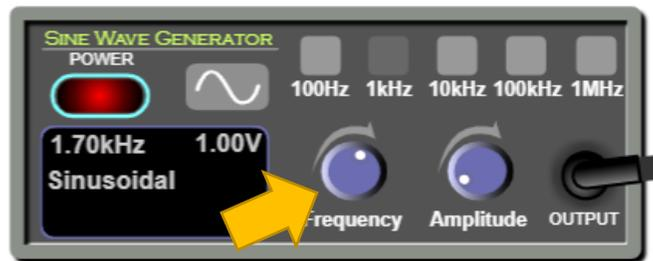
*Frequency ranges:* You can select a range so you vary the frequency accordingly using the frequency knob.
