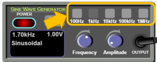
*Amplitude knob:* You can rotate this knob to vary the value of the amplitude of the signal.
