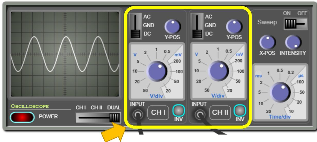
*Inputs:* Each channel has an input where you can connect the probe.
