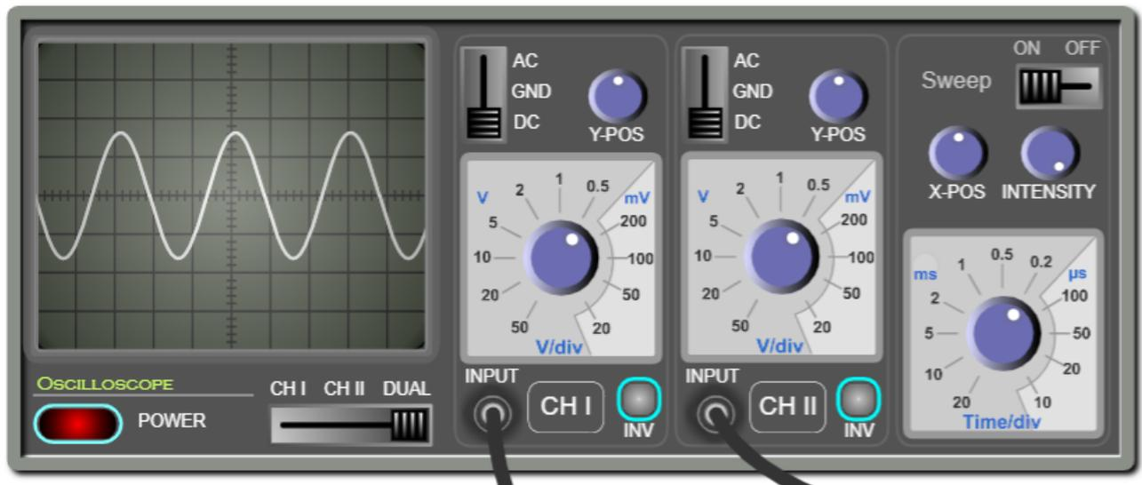
*ON/OFF switch:* This is used to turn on or off the oscilloscope.
